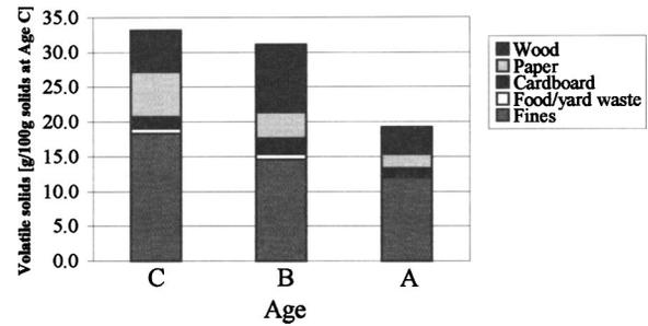
**Fig. 4.** Volatile solids mass of sample at various ages that consisted of 100 kg dry solids at Age C
