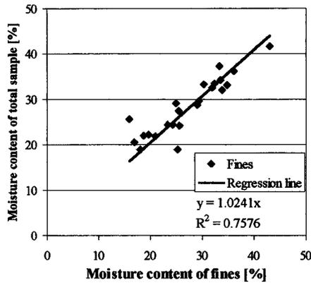
**Fig. 3.** Relationship between moisture content of fines fraction and total sample
