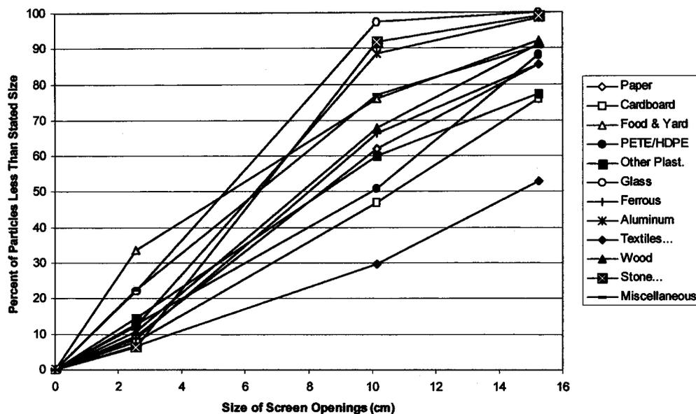
**Fig. 5.** Particle size of selected fractions
