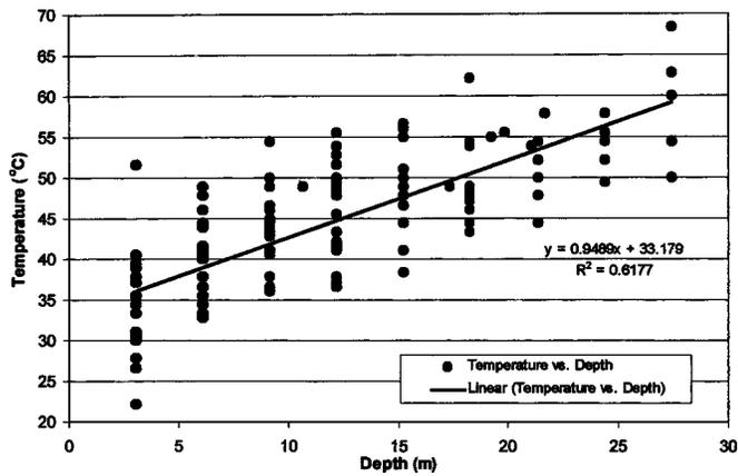
Fig. 1. Temperatures in landfill depending on depth
