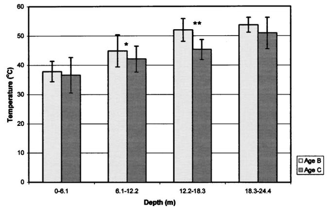
Fig. 2. Temperatures in landfill at Ages B and C
