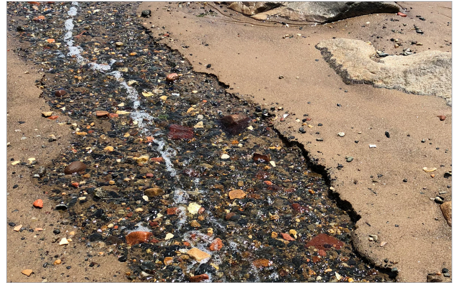
Figure 20. Sediment within the contract limit line is dominated by upriver silt and clay fractions. Courtesy of CUES.
