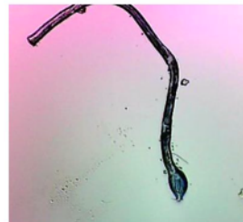
Blue fiber was woven in left over protein residue on filter. Removed and rolled out on Low-e. Identified as polyethylene terephthalate.
